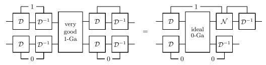
Property wGa3 says that, for a 1-Ga containing no faults, if the second output block is projected to the code space, then one error in the first input block does not propagate badly through the 1-Ga and cause an encoded error in the second output block. Similarly (though this is not illustrated by the diagram), one error in the second input block does not cause an encoded error in the second output block.
