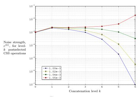
Fig. 24. The effective strength  $\varepsilon^{(k)}$  of locally correlated stochastic noise for level-k postselected CSS operations, as a function of k, for various values of the physical level-0 error probability  $\varepsilon$  (shown in the legend). The plot demonstrates that the threshold error probability is above  $1.04 \times 10^{-3}$ .
