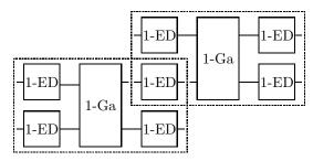
Fig. 3. Two consecutive level-1 extended rectangles (indicated by dashed lines). Each 1-exRec consists of a gate gadget (denoted 1-Ga) that realizes an encoded two-qubit gate, preceded by "leading" error detection gadgets (1-EDs) applied to each input block and followed by "trailing" error detection gadgets applied to each output block. The 1-exRecs overlap — a trailing 1-ED of the earlier 1-exRec is also a leading 1-ED of the later 1-exRec
