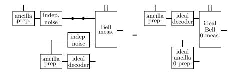
In the diagram, the double-line input and output to the Bell measurement indicates the classically recorded logical Pauli operator which is updated when Clifford-group gates are teleported. The circles on one input wire of the Bell measurement indicate the two storage steps that must be included if the previous gate is non-Clifford, in which case the outcome of the previous Bell measurement is needed to determine what ancilla state to use for the current gate.
