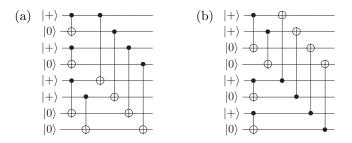
Fig. 13. Two encoding circuits for the logical Bell state  $|\Phi_0\rangle_L$ . In (a), the first block is prepared in the state  $|+\rangle_L|0\rangle_T$  and the second block is prepared in the state  $|0\rangle_L|+\rangle_T$ . Then, the transversal CNOT gate creates a logical Bell state while preserving the state  $|0\rangle_T|+\rangle_T$  of the gauge qubits. In (b), the two code blocks are interchanged, so that the gauge qubits are prepared in the state  $|+\rangle_T|0\rangle_T$ .
