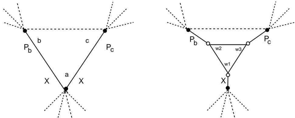
Fig. 5. Triangle Gadget. We first subdivide edges  $ab$  and  $ac$  and then apply the Fork gadget on vertex  $a$ . This give rise to a ‘mediator triangle’ such that vertices  $b$  and  $c$  have the same degree as before and vertex  $a$  has reduced its degree by 1.
