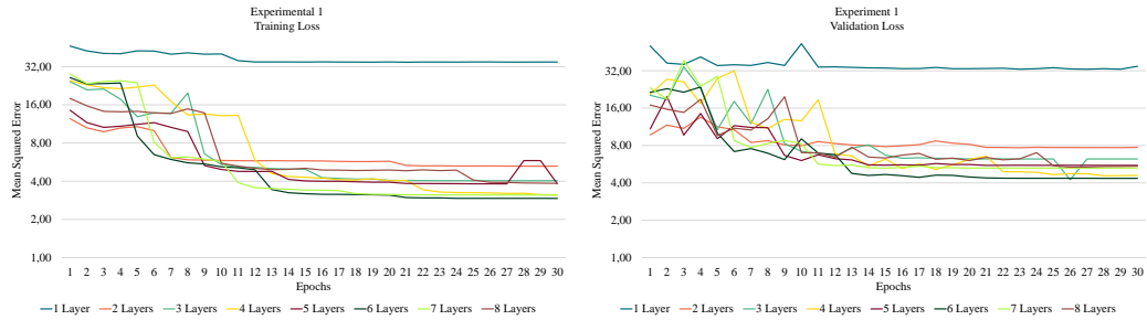
Fig. 9. Variation of training loss and validation loss for Experiment 1 with respect to the number of training periods.
