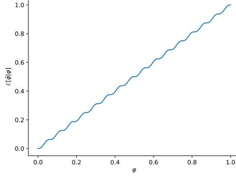
Fig. 2. The theoretical expectation of  $\tilde{\varphi}$  deduced from Eq. (3) in which  $T = 16$ , when the ground truth is  $\varphi$ . An unbiased estimation should satisfy  $\mathbb{E}[\tilde{\varphi}|\varphi] = \varphi$ .
