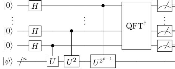
Fig. 1. The quantum circuit of PEA.
