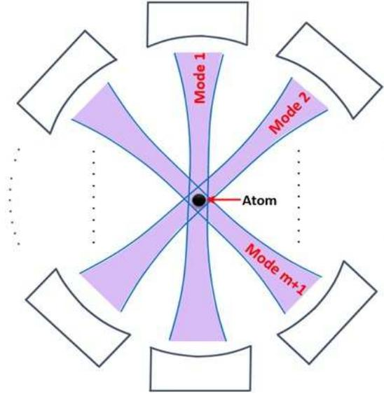
Fig. 1. Layout of the  $m$  modes cavity with  $\omega_i = \omega$  ( $i = 1, m$ ). A single two-level atom enters a multi-mode cavity and interacts with the photonic qubits present. The atom acts only as an ancilla.
