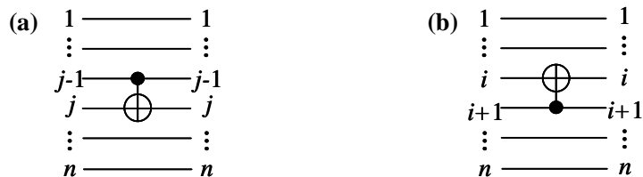
Fig. 9. (a) denotes a LNN CNOT-down gate. (b) denotes a LNN CNOT-up gate. Both (a) and (b) are CNOT gates located in n -line circuits.
