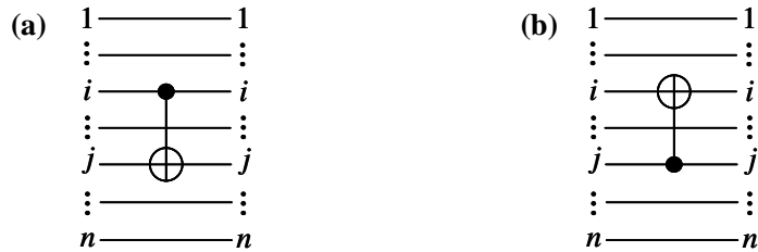
Fig. 8. (a) denotes a CNOT-down gate.(b) denotes a CNOT-up gate.Both (a) and (b) are CNOT gates located in n -line circuits.
