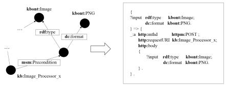
Fig. 4. A Linked Data-Fu rule for the Linked image converter.
