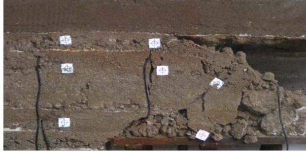
Figure 8 Sub-level coal's displacement failure situation of similar analogy experiment when Sub-level coal thickness is 12.8m
