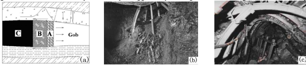
Figure 1 Scheme of damage regions in coal seam and gateroads after coal bumps in Tangshan mine. (a) Scheme of damage regions. A- pressure relief zone B- maximum static equilibrium zone C- primitive overburden pressure zone. (b) , (c) Gateroads after coal bumps.
