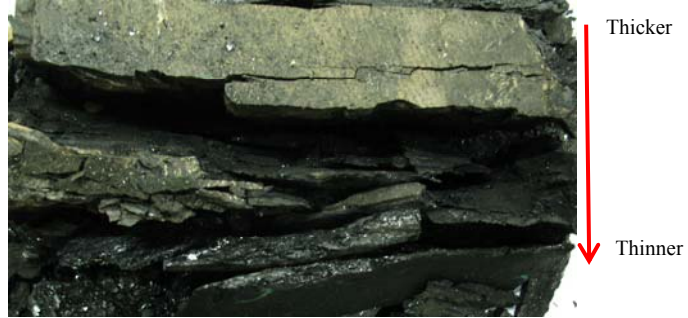
Figure 2. A series of fracture layers at which the thicknesses progressively varied after coalburst.
