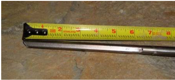
Figure 2 End of a yielded Roofex bolt. The initially round steel tendon has been cold rolled into a hexagonal shape as it was pulled through the energy absorber
