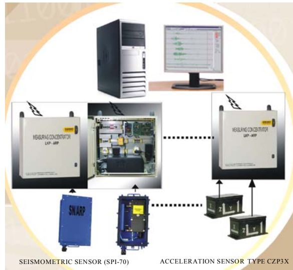
Figure 8 Shows ARP 2000P/E system structure with one component acceleration probes.
