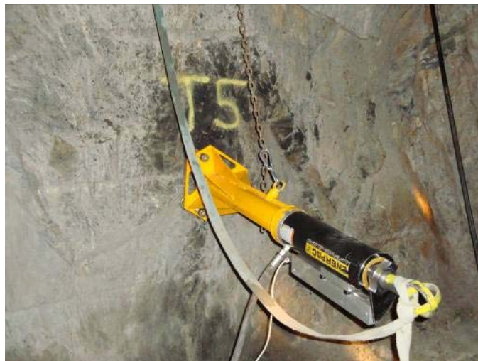
Figure 4 Tripod and ram pull test assembly at Edgar Mine.
