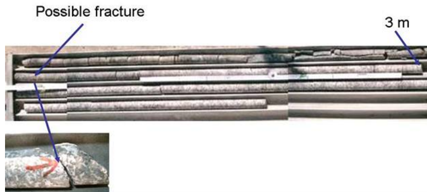
Figure 6 Borehole core and a possible fracture position at 1.6 m above the stope.
