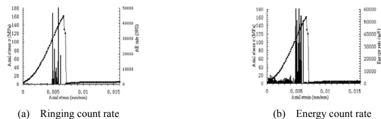
Figure 1 Test results of acoustic emission under uniaxial compressive condition of sandstone sample of Xinhe No.3 coal roof
